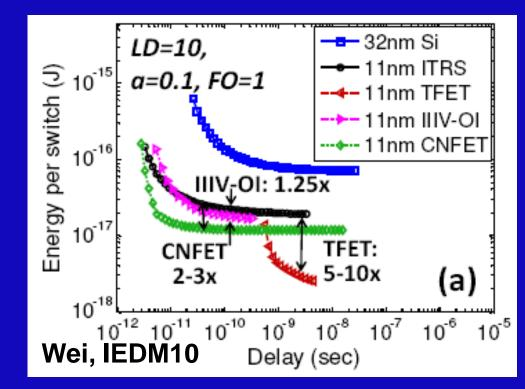
But, even if new switch only improves energy at higher delay (higher R<sub>on</sub>)...
