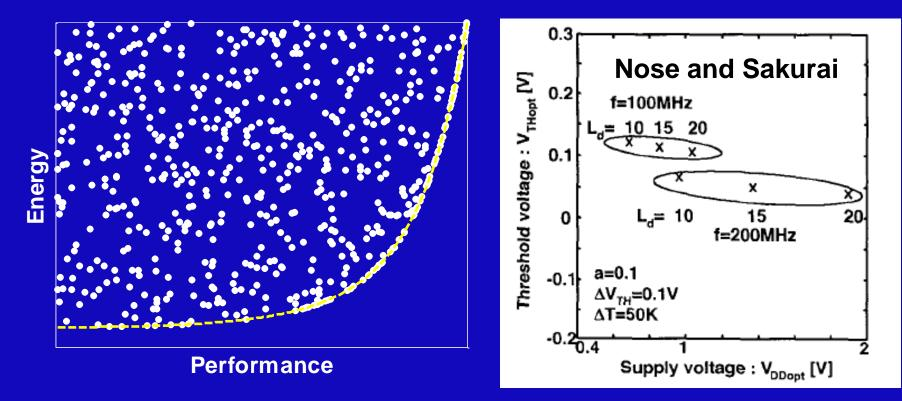
Pick V<sub>dd</sub>, V<sub>th</sub> to minimize energy for given performance (1/delay)
