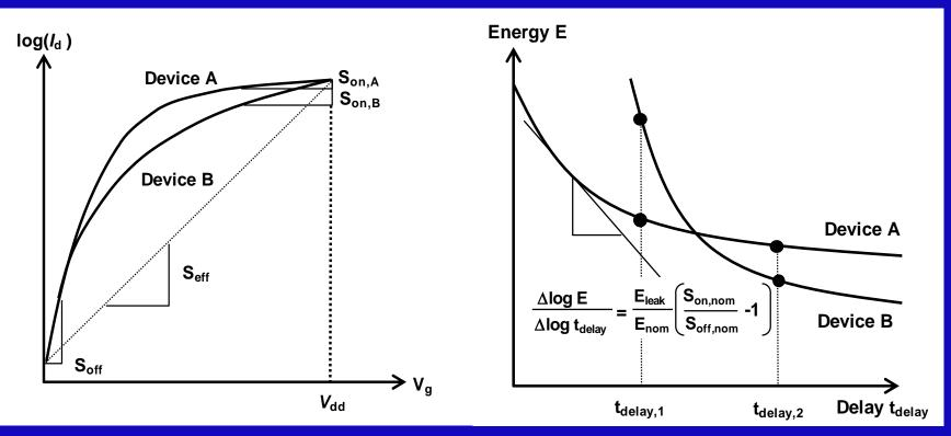
$$\frac{I_{on}}{I_{off}} = \beta \frac{L_d f}{4\alpha}, \quad \beta = -\frac{S_{eff}}{S_{off}} lambert W \left( -\frac{4\alpha}{L_d f} \frac{S_{off}}{S_{eff}} e^{\left(\frac{Soff + Son}{Seff}\right)} \right)$$
